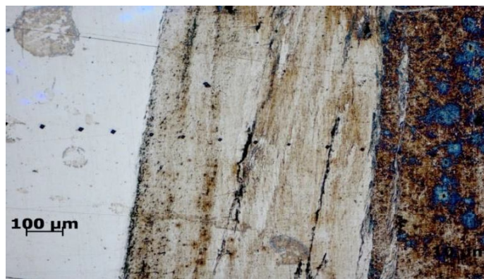
Figure 3,a - The optical micrograph of the weld zone area
