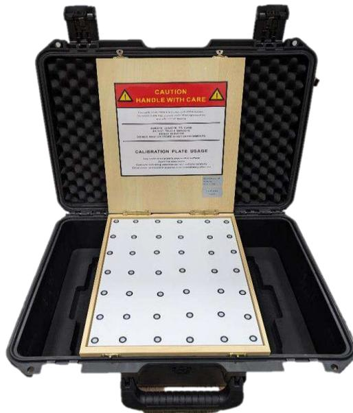
Figure 3 – Calibration Plate
