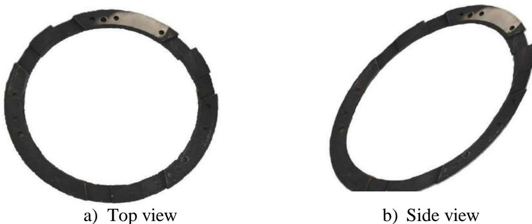
Figure 1 - Tool Change Mechanism Compensator
