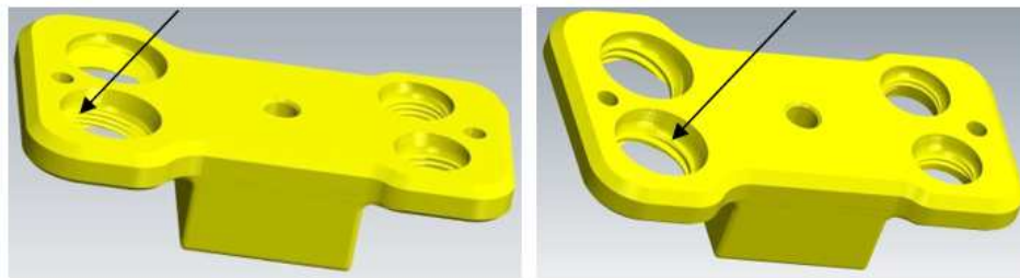
Figure 6: Simulation of Implants with One-Way and Two-Way Internal Thread: a) One-Way Thread; b) Two-Way Thread
