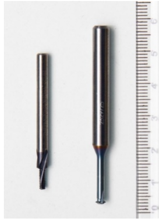
Figure 7: Left - Threading Tap for Single-Thread, Right - Special Threading Tool for Two-Thread
