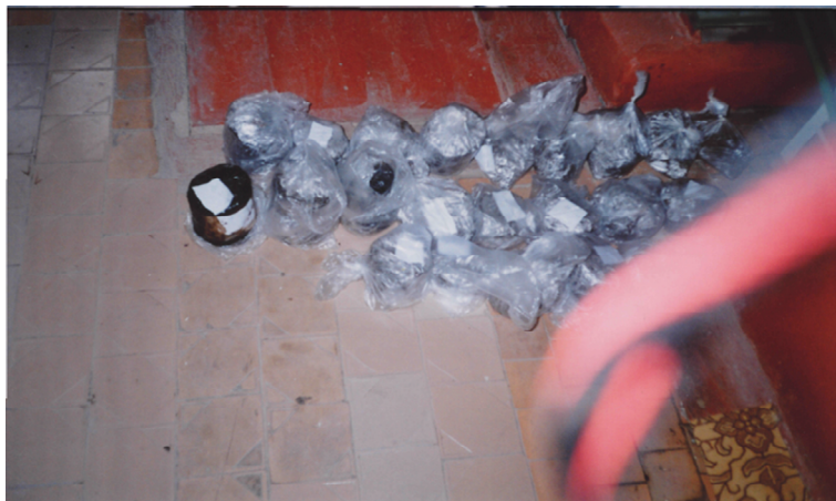
Figure 12 – Earth samples rolled up in gauze and flooded with paraffin.
